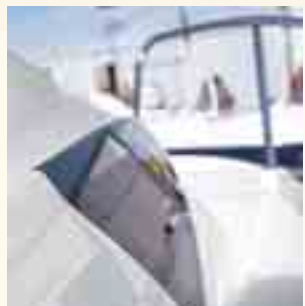
510 Cruiser. The automotive-style windshield is bonded in to keep out possible leaks.
